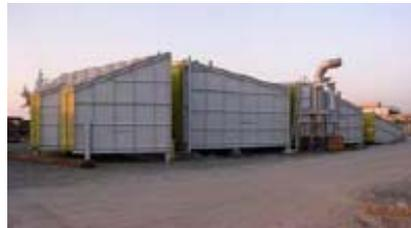
This modularized fired heater consists of 2 trains, the Steam Superheater and the Feed Gas Superheater, each with individual radiant and convection sections, and a common WHRU and stack. The Steam Superheater radiant and convection coils are fabricated in accordance with and stamped with the ASME "S" stamp.
