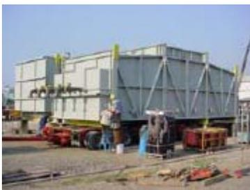
As part of a plan to replace aging equipment at its New South Wales refinery, Caltex called on Foster Wheeler Fired Heaters to supply a large crude oil VC heater.
