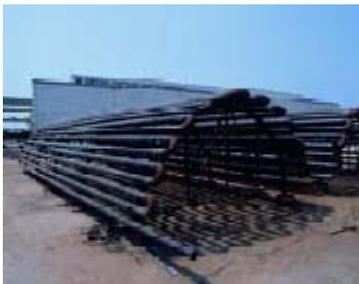
Each of the heaters' radiant sections were completely assembled at the Unithai's factory prior to delivery with radiant coils (2no. of SS321 stainless steel and 3no. of A-106 carbon steel) and internal ceramic fiber lining installed.
