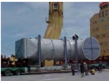
ABB LHT chose Unithai to fabricate and supply the heater, comprising of P9 radiant coil, 30 no.24 meter long unlined radiant panels, concrete lined ducting, a concrete lined stack,
