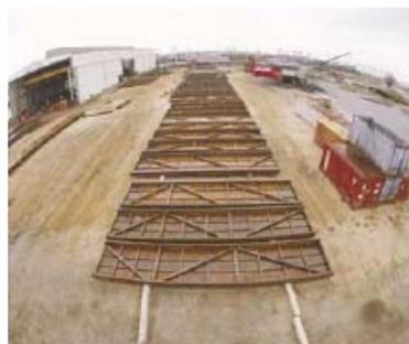
Unithai's scope of works covered the fabrication of radiant section steelwork for a pair atmospheric and a pair vacuum column feed heaters. Each pair of heaters shared a common stack.
